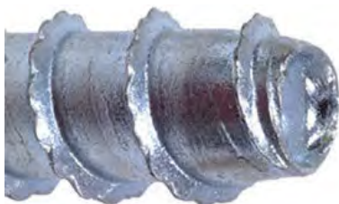
Serrated teeth on the tip of the Titen HD® screw anchor facilitate cutting and reduce installation torque.
