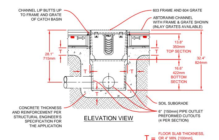
NOTE: YOU ARE NOT LIMITED TO THE OUTLETS SHOWN. OUTLETS AS LARGE AS 12" [300mm] MAY ALSO BE CUT OUT ON ANY OF THE SIDES OF THE 610 CATCH BASIN.
