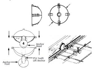
Warning: The P54 recess plug is designed to be used with the P52 insert and P59 shear bar combination.
